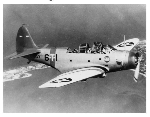
The **Douglas TBD Devastator** was an American <u>torpedo bomber</u> of the <u>United States Navy</u>. Ordered in 1934, it first flew in 1935 and entered service in 1937. At that point, it was the most advanced aircraft flying for the Navy, being the first <u>metal monoplane</u> in the <u>United States Navy</u>[1]; however, by the time of the <u>US entry into World War 2</u>, the TBD was already outdated.
