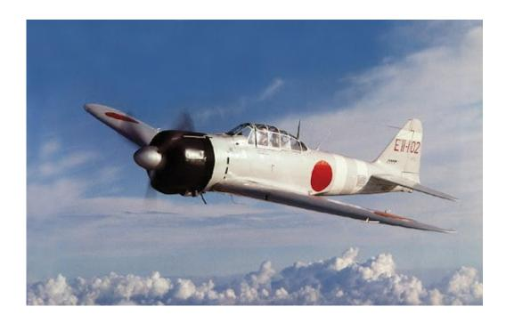
The **Mitsubishi A6M** "**Zero**" is a long-range <u>carrier-based</u> <u>fighter aircraft</u> formerly manufactured by <u>Mitsubishi Aircraft Company</u>, a part of <u>Mitsubishi Heavy Industries</u>. It was operated by the <u>Imperial Japanese Navy</u> (IJN) from 1940 to 1945. The A6M was designated as the
